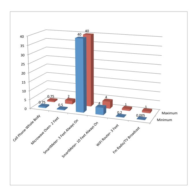
Figure 4. Comparison of Radio-Frequency Levels to the Whole Body from Various Sources in  $\mu$ W/cm<sup>2</sup> over time [corrected for assumed duty cycle and whole body exposure extrapolated from EPRI/CCST SmartMeter estimated levels at 3 feet].
