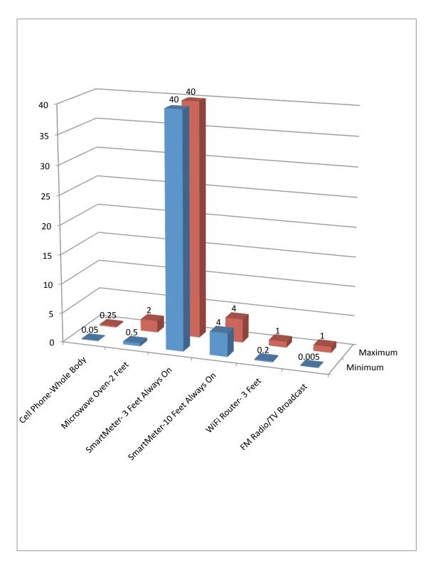
Figure 3. Comparison of Radio-Frequency Levels to the Whole Body from Various Sources in  $\mu$ W/cm<sup>2</sup> over time [corrected for assumed duty cycle and whole body exposure extrapolated from assumed cell phone dose at ear].
