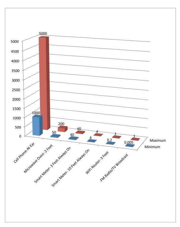
Figure 1: Graph from CCST Report in  $\mu\text{W/cm}^2-\text{uncorrected}$  for whole body exposure or duty cycle
