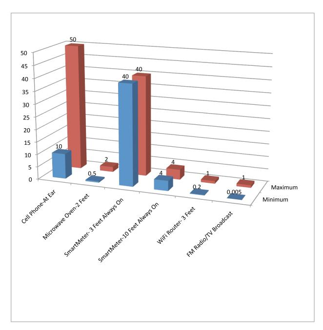
Figure 2. Comparison of Radio-Frequency Levels from Various Sources in  $\mu$ W/cm<sup>2</sup> over time [corrected only for assumed duty cycle].
