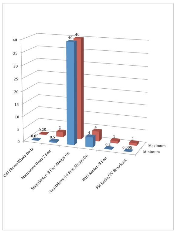
Figure A. Comparison of Radio-Frequency Levels to the Whole Body from Various Sources in  $\mu$ W/cm<sup>2</sup> over time [corrected for assumed duty cycle and whole body exposure extrapolated from assumed cell phone dose at ear].
