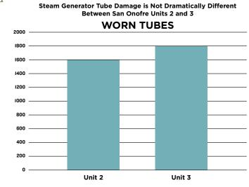
service) 510 tubes, whereas Unit 3's fever is slightly higher, The data tables posted by NRC show similar numbers of damaged tubes in the two units. Unit 2 has 1,595 tubes with wear, Unit 3 has 1,806.
