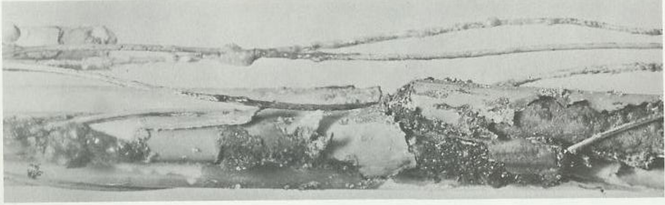
Figure IV-A-7. Midsection of Damaged Element in Channel 55
