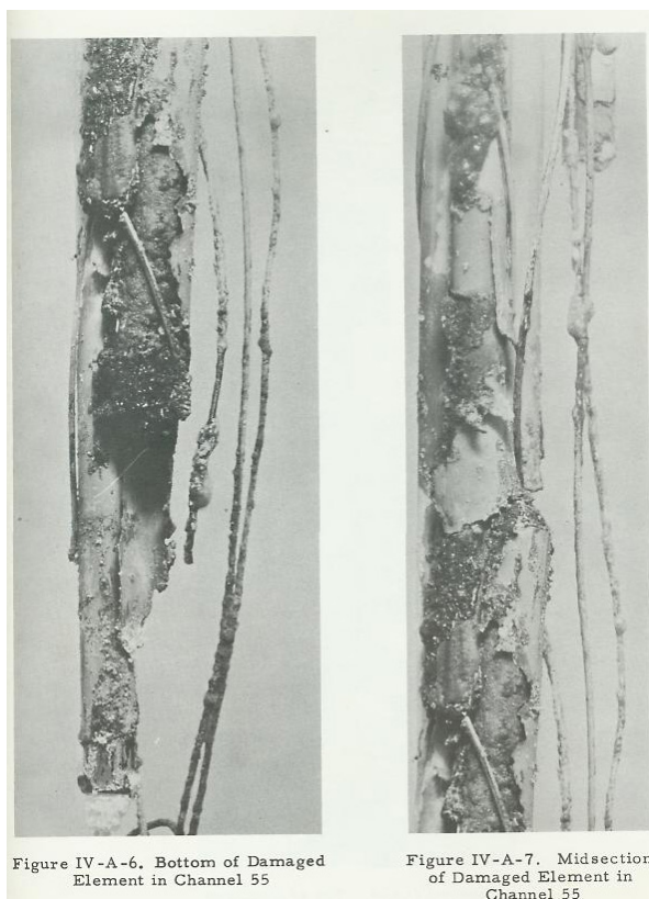
Photo of Damaged Fuel Element; source: AEC/Atoms International
